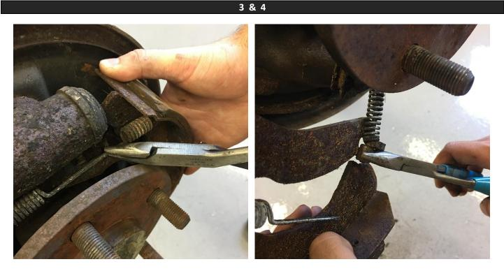
Remove the additional retaining springs from the brake shoes. Disconnect the parking brake cable from the brake shoe, then remove and discard the brake shoes and hardware.
