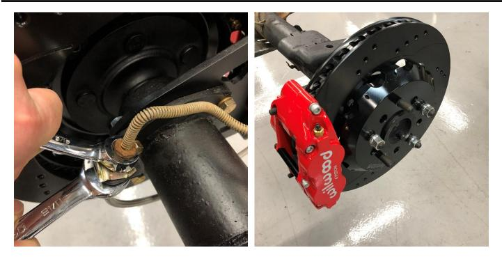
If you do not plan on installing new brake lines, the factory brake line can then be rerouted and tightened into the stainless hose. It is best to use a wrench to support the stainless hose from spinning in the hose bracket.
