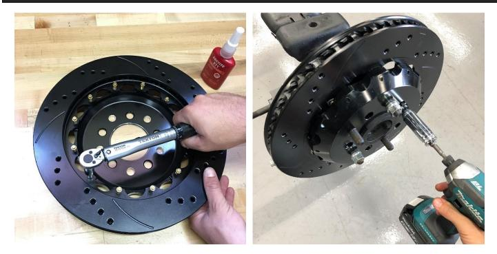
Arrange the rotor and hat in the position shown ensuring the arrow noting rotation direction is correct for its position on the vehicle. Start the first few threads of all 12 of the ¼-20 12-point bolts. Using an alternating sequence, apply red Loctite<sup>®</sup> 271 to the threads, and torque to **155 in-lbs**. The rotor can be installed on the axle at this time using three lug nuts to hold the hat flat against the axle.
