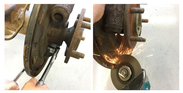
The 4 bolts retaining the drum backing plate to the axle can now be removed and discarded. The brackets in this kit are designed to be installed without removing the differential cover. This can be done by use of a cut-off wheel or reciprocating saw to split the drum backing plate into two pieces for removal. If you wish to retain your drum backing plates, the axles can be removed from the housing by draining the fluid, then removing the differential cover, cross pin, and C-clip retainers.
