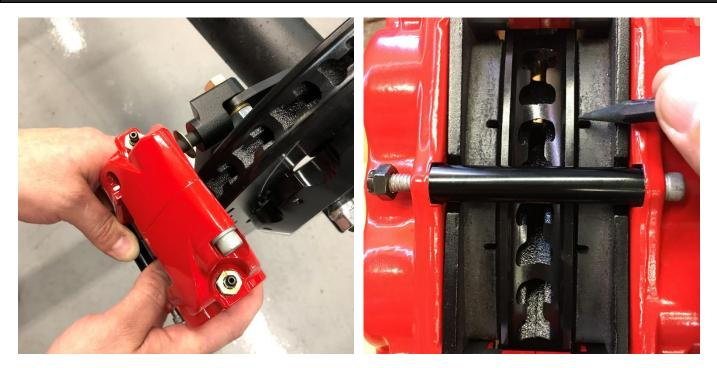
Lubricate the caliper mounting studs with lightweight oil. Initially place one .375x.875x.035 shim on each stud of the bracket. Mount the caliper using lock nuts and washers and ensure that it fully seats on the bracket and does not contact the rotor.
