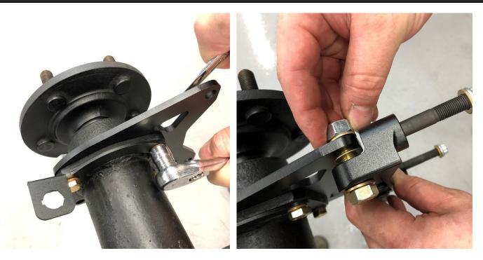
Bolt on the brackets using the supplied hardware, as shown. The calipers should be mounted to the **REAR** of the axle. The radial brackets can temporarily be installed at this time using the supplied 7/16 bolts and two .438 x .750 x .030 shim washers between the axle bracket and radial bracket. If you have the optional braided hose kit, the hose bracket will also be installed at this time as shown using the provided hardware.
