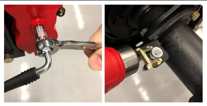
Install the stainless hose onto the caliper fitting. The hose will be routed under the axle and through the hose bracket. Install the retaining clip as shown, being careful not to bend the hose bracket.
