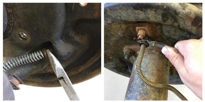
The cable can then be removed from the backing plate by depressing its perimeter springs. Remove the brake line from the wheel cylinder using a line wrench if possible.
